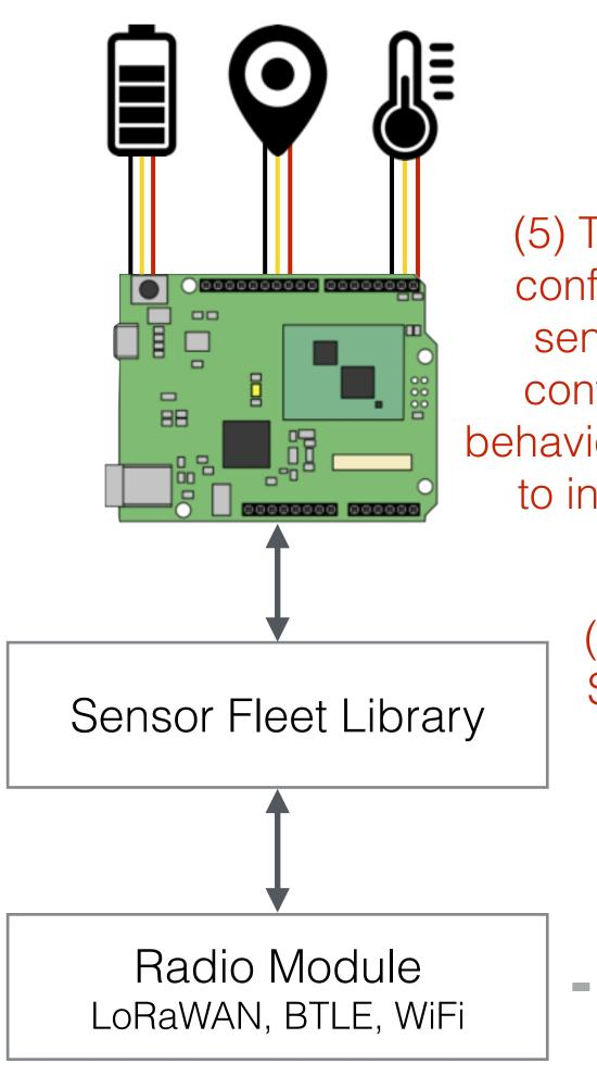
(5) The device configures the sensors and configures its behavior according to instructions
